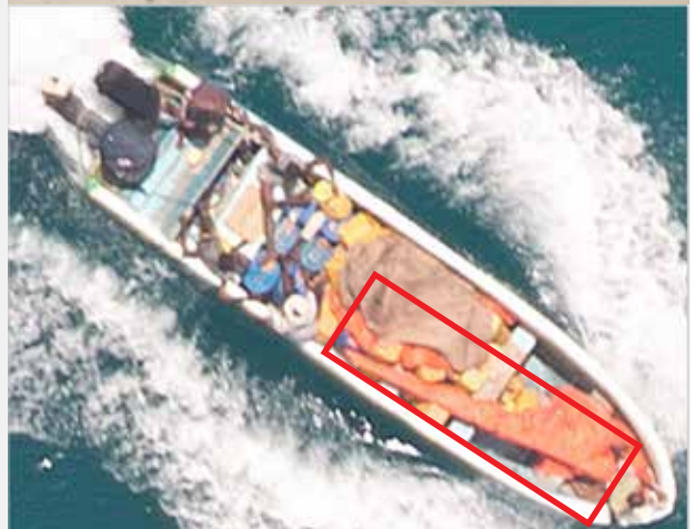
Maritime Patrol & Reconnaissance Aircraft took this image of a pirate skiff in Summer 2013. In the second image the skiff has been deployed to look for target of opportunity. Highlighted in the red box is a 3.5 metre ladder used to board high sided Merchant Vessels, it is clearly visible.
